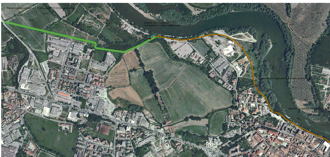
Figure 3.28: Position of the levees that complete the protection of Lodi town.
